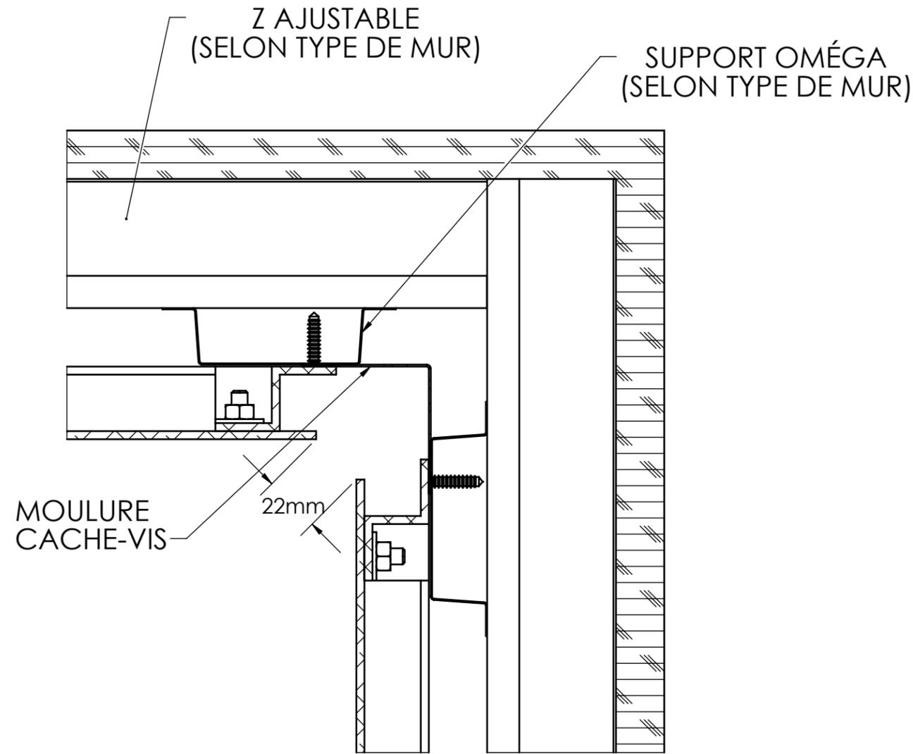
DÉTAILS COIN INTÉRIEUR AVEC JOINT
